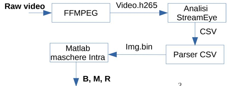
$$I_{mask} = w_b \cdot B_{mask} + w_m \cdot M_{mask} + \sum_{i=1}^3 w_i \cdot R_{mask}^i$$
