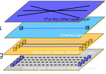
OAM layer in short-distance links inside data centers: avoid MIMO processing, ACDs, ultra-fast DSP
