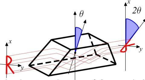
A rotated Dove prism inverts and rotates of  $2\alpha$  any incident image
