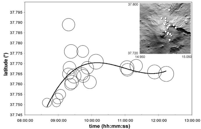
**Figure 6.** Location of the seismic swarm preceding and accompanying the onset of eruption on 13 May 2008 plotted as function of latitude versus time. The size of the circles is proportional to the duration magnitude ( $M_{Dmin} = 1.0$ ,  $M_{Dmax} = 3.3$ ). The line is a fourth-order polynomial curve fitting the data set. Inset shows the map of the summit area with the position of the epicenters.
