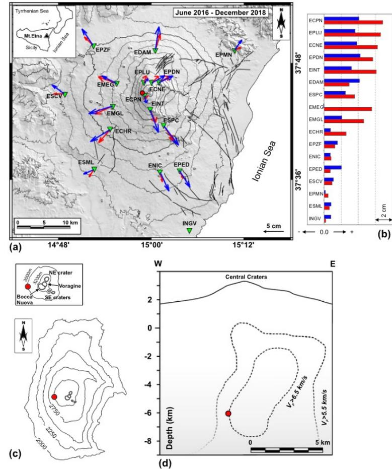
**Figure 1.** (a) Recorded (blue) and modeled (red) deformation pattern at Mount Etna during the recharge phase before the December 2018 eruption (June 2016 to December 2018). The histogram (b) reports the recorded (blue bars) and modeled (red bars) vertical displacements. The vertical variations are plotted according to the CGPS station elevations. Horizontal and vertical projections (c, d) of the modeled inflation source are reported.
