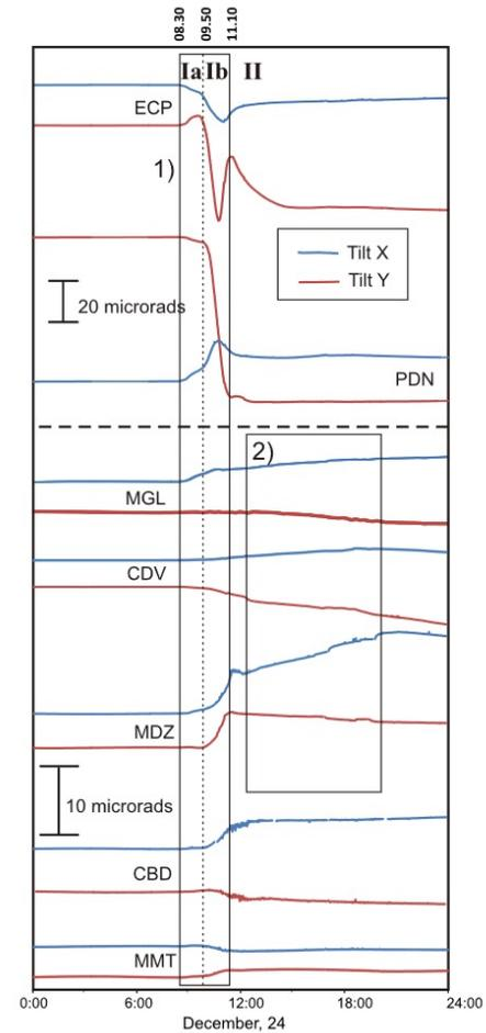
Figure 3. Tilt components recorded on 24 December 2018 at selected stations. (1) 8:20 and 11:10 UT interval where ECP and PDN recorded the strongest variations; (2) period after the 12:00 UT when significant tilt changes were recorded at the southern stations.
