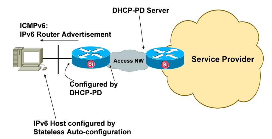
IPv6 Addresses Configured Dynamically by DHCP-PD
