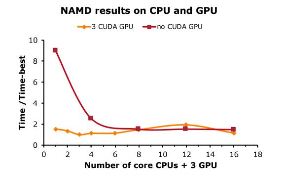
Preliminary results using a 16 cores + 3 TESLA GPU machine
