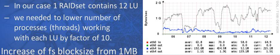
Cache throughput to 4MB has reduced I/O operations to get same throughput (and also reduced concurrent I/O on a specific RAIDset)
