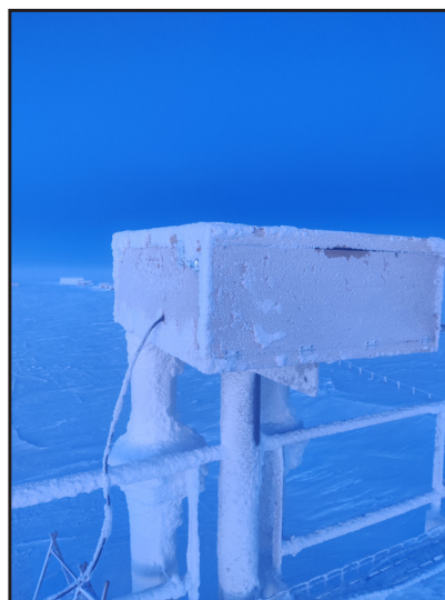
Fig. 6 Insulation enclosure at -70^{\circ}\text{C}
